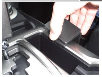
1. Use the enclosed alcohol pad to clean the area where the ProClip is to be installed. Peel off the cover of adhesive tape on the ProClip. Note: The adhesive tape does not leave any marks or damage the dashboard, and it is easy to remove. Place the ProClip in your hand so the ProClip label (sticker) is in an upright position, or if vertically positioned; the P in ProClip is at the top. Place the angled edge on the left side of the ProClip over the console edge.
