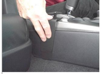
2. Place your finger on the top right side of the ProClip and press firmly down so the ProClip flexes towards the carpet and hooks around the console edge.
